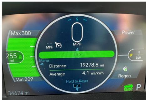
The displays in electric vehicles inform drivers of the status of the battery and estimated driving range along with other information on the car's performance.
