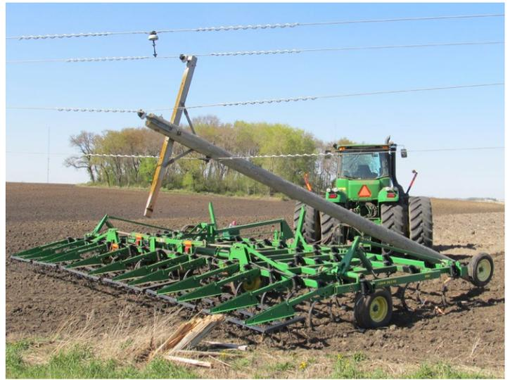
If your equipment does make contact with a power line, do not leave the cab. Immediately call 911 to have the utility notified. Warn others to stay away, and wait for the utility crew to cut the power. Never try to disentangle equipment on your own.
